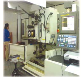
• CNC WIRE CUT CALIBRATION BY LASER
